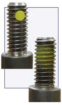
Conforming bolt and nonconforming bolt; the conforming one contains the yellow self-locking pellet. The nonconforming one has a yellow sprav mark.
