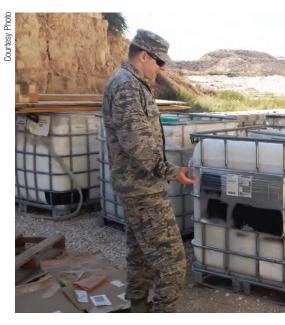
An Army and an Air Force engineer review a pallet of containers of DLA-provided groundhardening paste, commonly called "rhino snot," which is used to reduce dust. This shipment was used to coat a makeshift runway for an unmanned aerial system.
